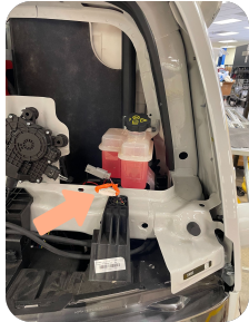
High voltage interlock loop (orange) under the front cap
