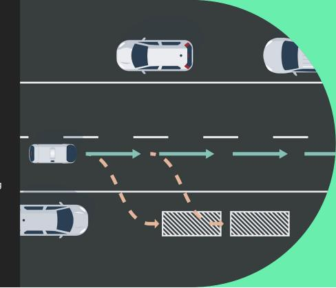
If some component in the vehicle is not operating as intended, we must be able to detect it and respond safely. Our approach is to use redundancy and layered fallback safety strategies, so that we can maximize safety even if something goes wrong under challenging circumstances. Nuro's onboard systems check for faults hundreds of times per second, ensuring all systems are operating safely, and take action if needed.
