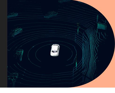
Recording what is happening in and around our vehicles powers the machine learning that enables continuous improvement of the self-driving software. By capturing details from our real-world drives, we can evaluate system performance and build simulations to practice challenging situations, ultimately building a more capable self-driving vehicle. Nuro can then apply the learnings from any one of these vehicles to the entire fleet to improve safety and efficiency.
